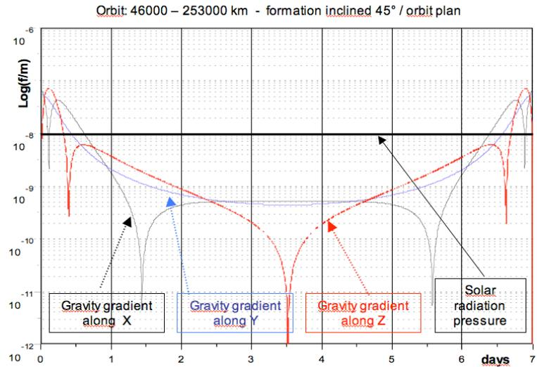
**Figure 6 :** Comparison of the solar radiation pressure with the gravity gradient along the 7 days of the Simbol-X orbit, for the 3 spatial axes.
