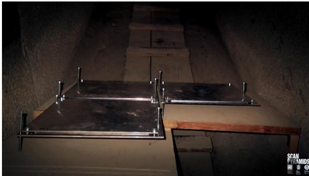
Image 11 - Nagoya University Muon sensitive plates in descending corridor that have been analyzed
