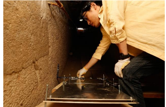
Image 12 - Nagoya University emulsion film setup in the descending corridor
